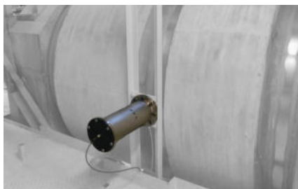
NHK for loosening adhesions on rotary kiln
