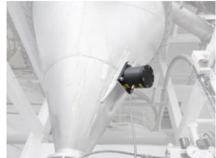
NTS 54/02 for improving material flow
