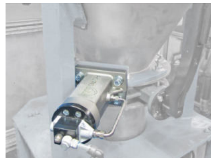
PKL 740 for loosening bridge formations
