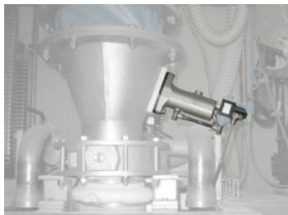
PKL 190 for improving material flow
