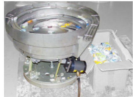
NTS 100/01 for spiral conveying of bulk materials
