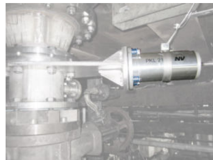
PKL 2100 for loosening adhesions
