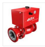
The Insulation System ExPinch is capable of isolating an explosion inside an equipment or container. The system needs to perform continuous monitoring of static and/or dynamic pressure sensors, that sends a signal to the line controller, activating a solenoid valve that releases the compressed air in a boiler which causes the immediate closure of the inner rubber sleeve.
